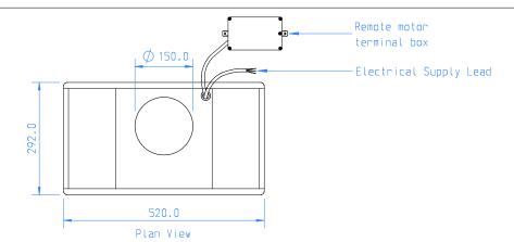
Sprung safety 135.0 250.0 clips x 2 Adjustable Spring Toggle x 4 280.0 51.5 320.5 Toggle Centres 494.0 520.0 Front View
