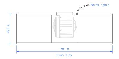
325.0 250.0 ∅ 150.0 Sprung safety clips x 2 Adjustable Spring Toggle x 4 280.0 694.0 Toggle Centres 874.0 900.0 Front View
