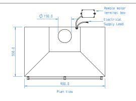
Motor: 1 x SEM Remote Motor - Separate Item
