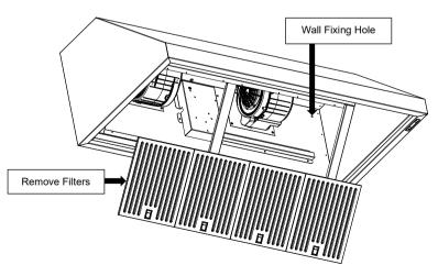
Once the filters have been removed, locate the wall fixing holes located at the rear bulk head of the appliance.
